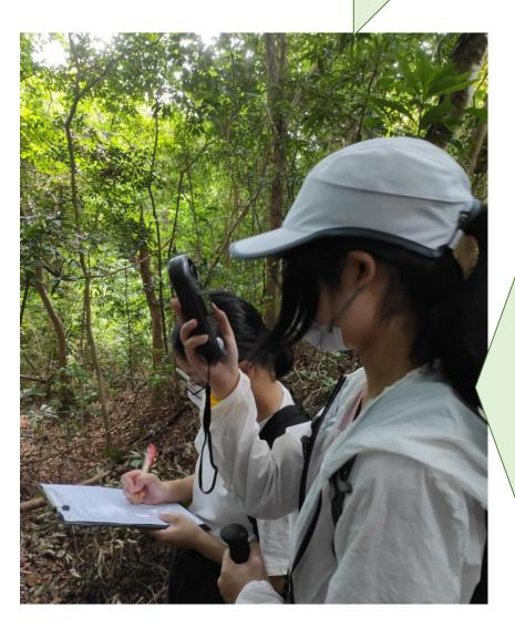
Students using anemometer to measure environmental parameters, including wind speed, light intensity, relative humidity and temperature.
